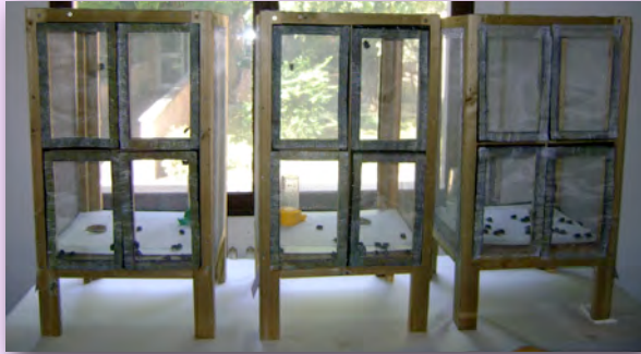
Flying cages made of wood and metal mesh, placed in front of a window to allow a natural light/dark cycle
